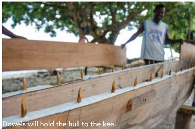
Dowels will hold the hull to the keel.
